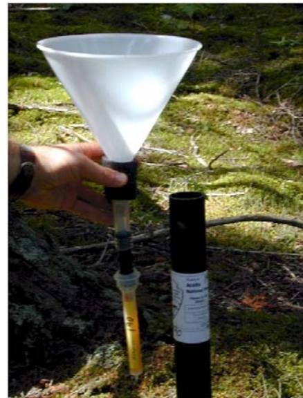
FIGURE 3. Bulk collector with ion exchange cartridge (Weathers et al., in prep) (do not duplicate without permission)
