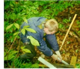
Driving 1 1/2" pipe to develop hole for lysimeter installation
